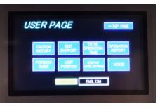
Easy to read, high-contrast, color touch screen for backup control and over 40 alert codes that can be visualized for service diagnostics.
